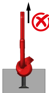
If the link remains in the position showed above, the lifting of the concrete unit is not allowed.
