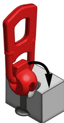
3 The link rotates to its locking position.
