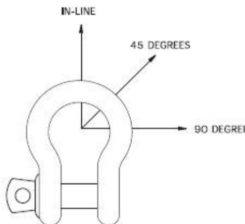
In-line loading is considered to be a load perpendicular to the pin and in the plane of the bow. Load angles in the table are the deviating angles from the in line loads. When using shackles in connection with multi-leg slings, due consideration should be given to the effect of the angle between the legs of the sling. As the angle increases, so does the load in the sling leg and consequently in any shackle attached to that leg.
