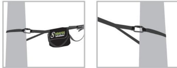
**IMPORTANT:** When there is no anchorage point, the forked ends of the lifeline allow inserting a structure. For this kind of installation, the lifeline straps should not be installed on sharp edges and have to be protected adequately. The connectors (EN362) used at the ends should be in steel and should never be in contact with the structure (pure tension between the two straps).
