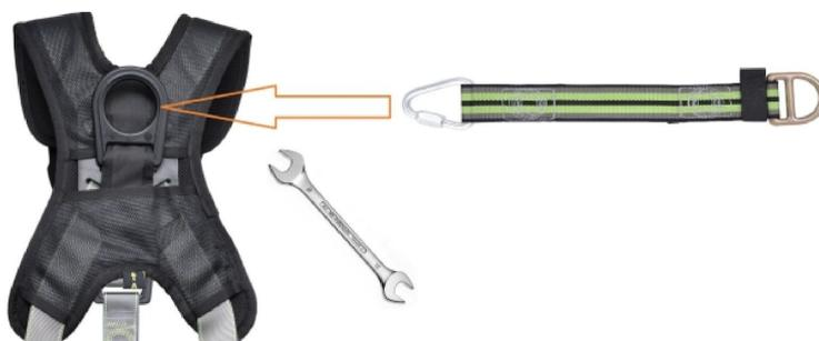
The extension lanyard FA 10 903 00 must be connected to the dorsal D-Ring of a full body harness (EN361) via the provided Delta quick link (EN362). The assembly shall be fitted tightly with a 14 flat key.
