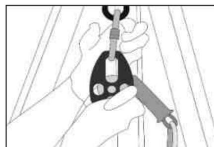
The handle of the fall arrester should be folded up before each use.
