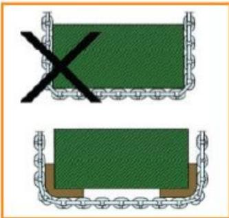
Tab 4. Working load variation depending on use of chain in contact with edges.
